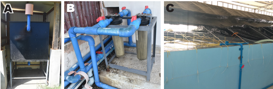
Figure 17. The aeration system: A. UV sterilizer, B. 0.45 \mu m cartridge filter, C. larval rearing tank with aeration
