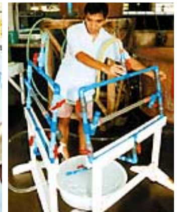
Apparatus used to test swimming performance of milkfish fry
