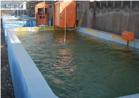
(Left) Tanks used to demonstrate the effects of higher water temperature on the reproductive performance of rabbitfish. Note the water heater (in orange on the right side) and the thermostat control for the heater (big orange structure at the end of the tank). Water is heated (29 - 33°C) and the temperature is automatically maintained by the thermostat (Right). The recirculating system set-up for the larval rearing experiments (milkfish, sea bass and rabbitfish) where the water temperature is again maintained by small heaters with thermostat
