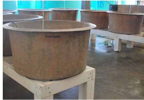
(Left) Tanks used to demonstrate the effects of higher water temperature on the reproductive performance of rabbitfish. Note the water heater (in orange on the right side) and the thermostat control for the heater (big orange structure at the end of the tank). Water is heated (29 - 33°C) and the temperature is automatically maintained by the thermostat (Right). The recirculating system set-up for the larval rearing experiments (milkfish, sea bass and rabbitfish) where the water temperature is again maintained by small heaters with thermostat
