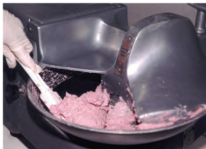
2. Mixing minced fish and other ingredients in silent cutter in a silent cutter
