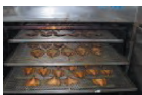
6. Hot air oven drying 40°C for 30 minutes
