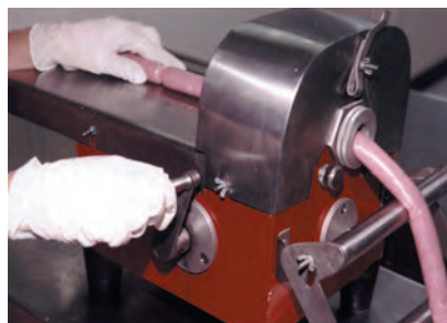
4. Clipping ('close') both end of the product using a clipping machine
