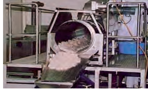
Continuous leaching using rotary sieve
