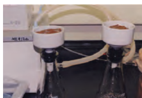
9. 2 nd filtration – vacuum filtering
