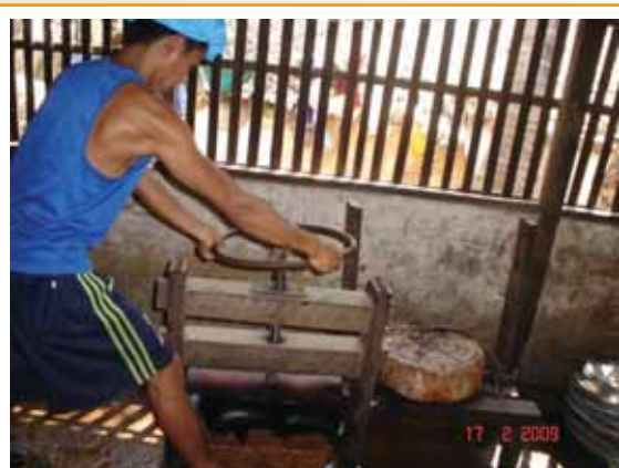
Figure 2 De-watering of ground/minced fish meat using screw press
