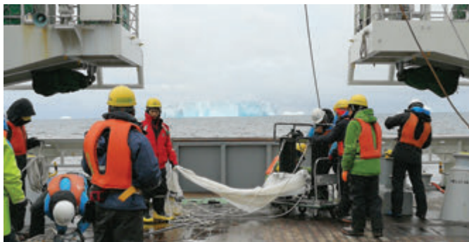
The biological group preparing the vertical multilayer plankton sampler for collecting plankton from depth 400 m to surface
