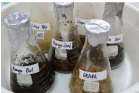
Bacterial treatment of selected agricultural wastes and by-products (ABPs) with Bacillus subtilis is explored to improve their nutritional composition
