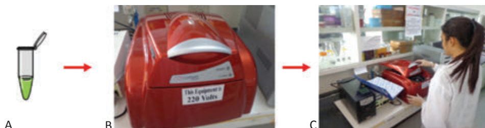
Optimization of q-PCR protocols: (A) Preparation of Master Mix with SYBR Fast q-PCR Master Mix (KAPABiosystems, USA); (B) Amplification carried out in Corbett Rotor-Gene 6000 Real-Time Rotary Analyzer (Corbett, Australia); and (C) Amplification program patterned from Optimized conventional PCR protocol
