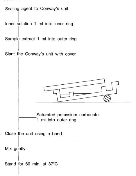
Titrate inner ring solution with 0.02N-HCl using a micro-burette
