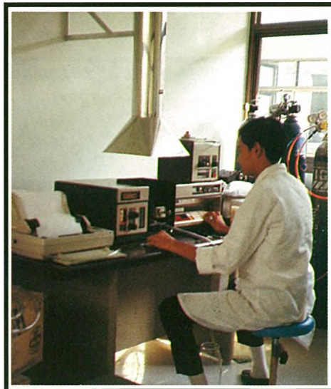
Determination for mercury using mercury analyser
