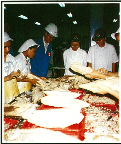
Loin cleaning operation in which time and sanitation should be controlled
