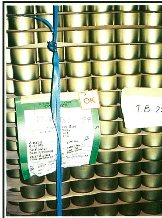
Every lot of empty cans should be inspected
