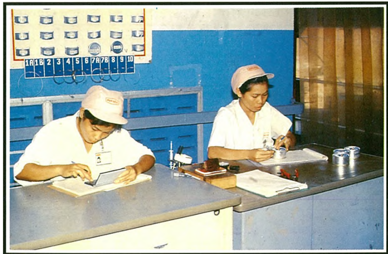
Seam tear down
