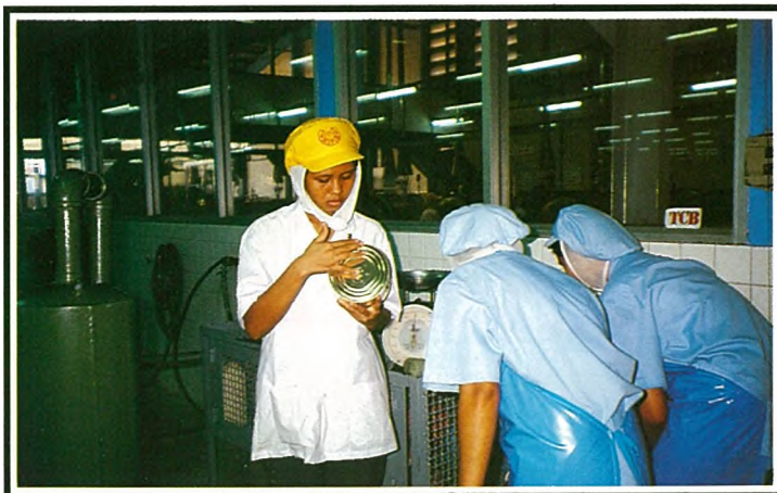
Visual inspection of seam
