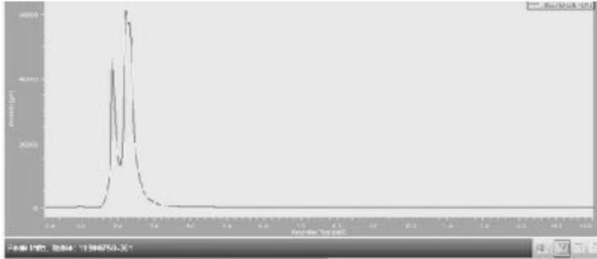
Figure 6. Sample chromatogram of a sample negative for domoic acid
