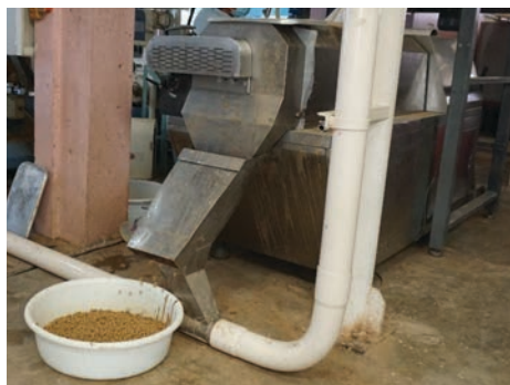
New extruder at AQD's feed mill for production of aquaculture feeds
