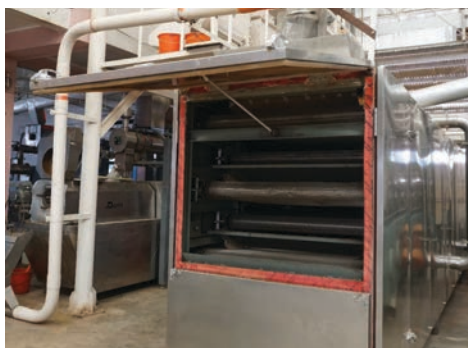
New 5-layer dryer replaces the ovens previously used to dry feeds at AQD's feed mill
