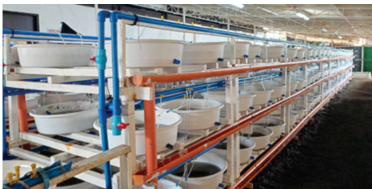
Modular tank setup for the grow-out culture of polychaetes
