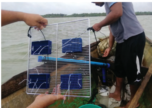
Passive sampling at Aparri using an improvised sampling grid with membrane filters
