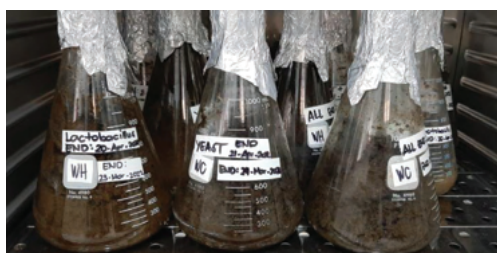
Two-stage fermentation process of aquatic weeds
