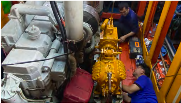
Installation and testing of the sherbet ice system on a purse seine fishing vessel in Pattani Province, Thailand
