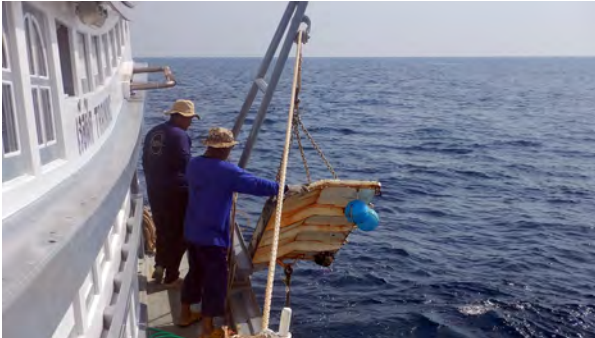
TD staff performing experiment on the comparative efficiency and impact of Vee type and rectangular flat otter boards for trawling onboard M.V. PLALUNG
