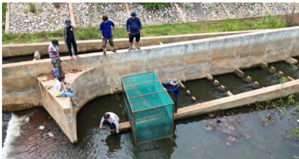
Staff from TD monitoring the effectiveness of fish passage at Huay Wang Chang Weir in Sang Khom District, Udonthani Province, Thailand
