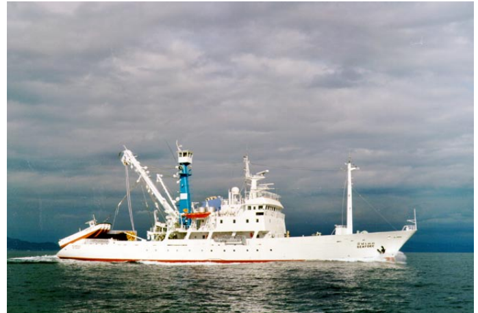
Fig. 3. The M.V. SEAFDEC (tuna purse seine research/training vessel) used by SEAFDEC/TD to conduct tuna purse seine operations in the Eastern Indian Ocean
