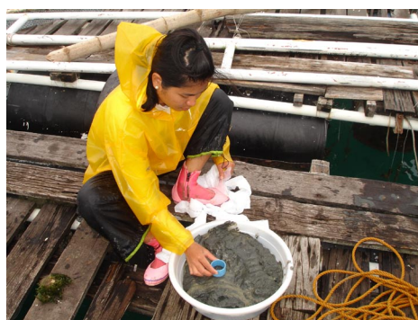
AQD’s program leader for aquatic ecology, Ms. Sheila Santander (below), assesses the sediment taken from AQD’s mariculture park by means of a core sampler. She does this to refine and make more detailed color chart on sediments that fish farmers can use. From top to bottom, good to bad to worse sediment
