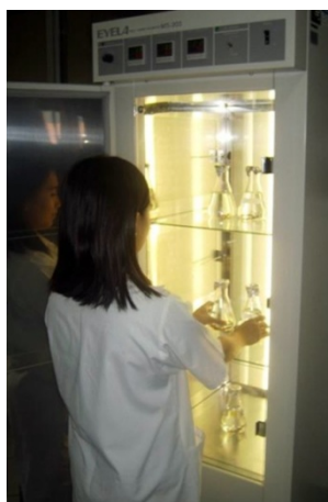
Tissue culture of seaweed ( Kappaphycus ) in a temperature gradient incubator facility at AQD
