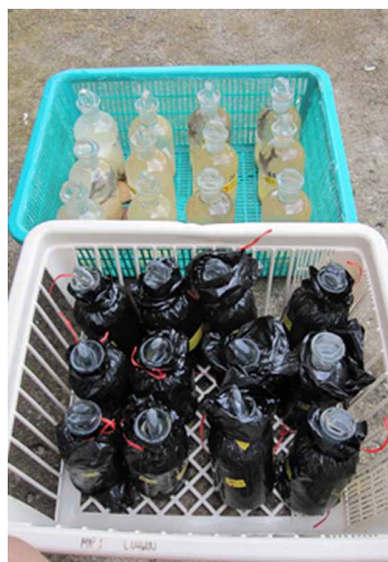
Effect of fertilization on the photosynthesis of K. alvarezii was determined using the 'Light and Dark Bottle' method
