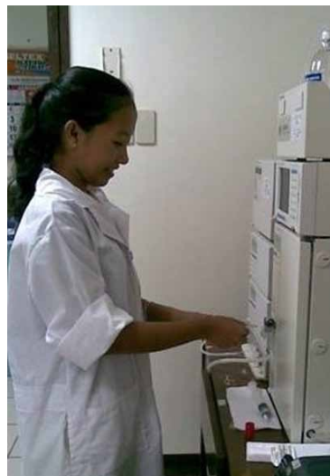
Detection of antibiotic residues in aquaculture products using the High Performance Liquid Chromatography (HPLC)
