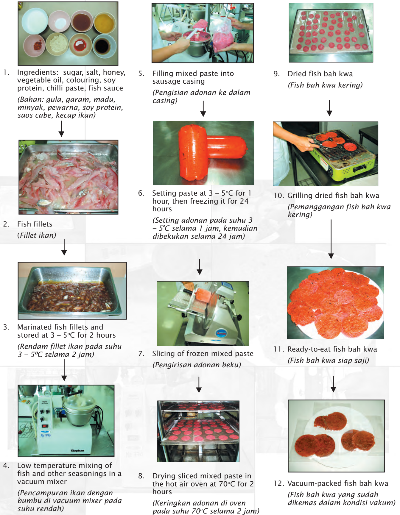
Fig 1.1. Illustrated flow chart of processing fish bah kwa Gambar 1.1. Ilustrasi skema proses pengolahan fish bah kwa
