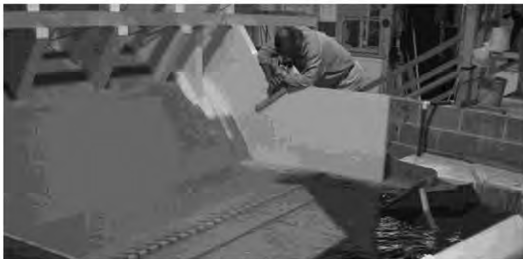
Figure 4. Example of a physical model of a 32 m high dam and fishway in Australia that was used to determine entrance location and hydraulic conditions for the fishway. Scale is 1:20 but 1:10 is preferred.
