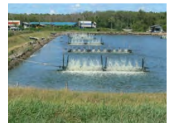
Figure 11. Ten 4-wheel aerators
