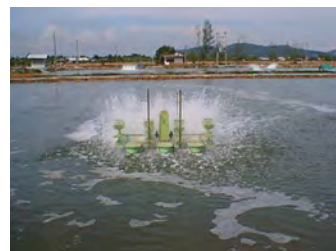
Figure 10. Typical 4-wheel aerator
