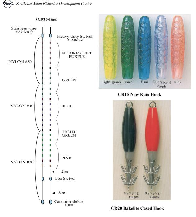
Fig. 2. Arrangement of squid jig line and types of squid jig used in the experiment.
