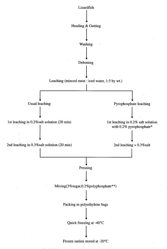
Fig. 2. Diagram showing the production of frozen surimi.
