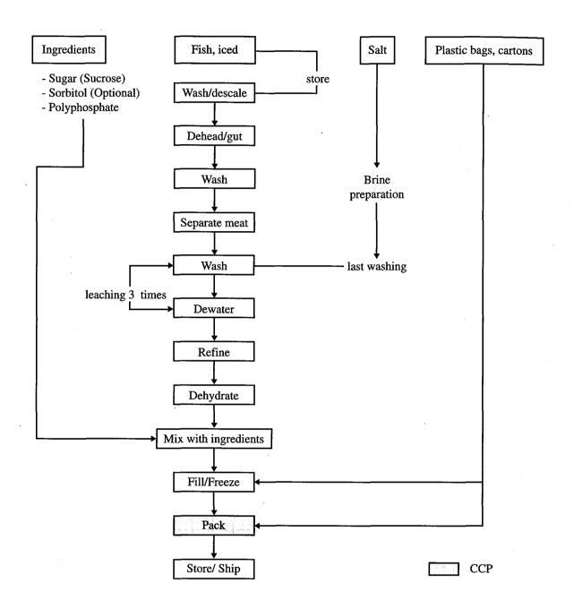
Fig. 1. Flow process diagram of frozen surimi.
