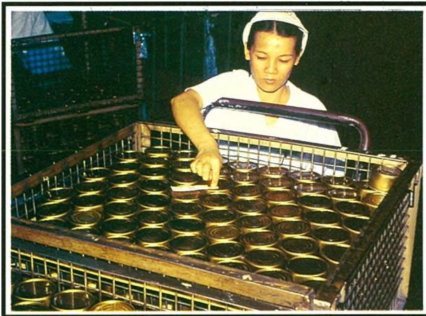
Heat sensitive indicator is used to ensure that cans passed heat processing, and will not mix with un-retorted lot
