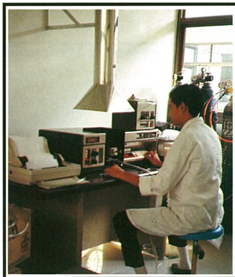
Determination for mercury using mercury analyser
