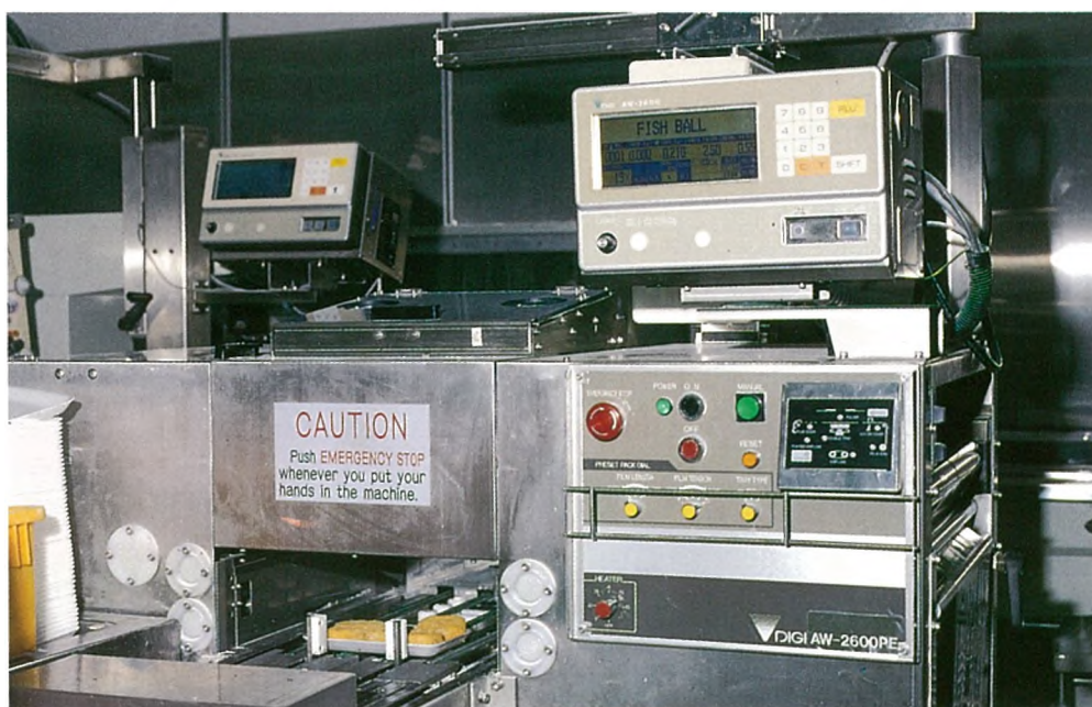
Figure 44. Automated shrink wrap equipment
