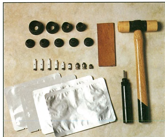
Fig.2 Tools for heat penetration study in retort pouch.
