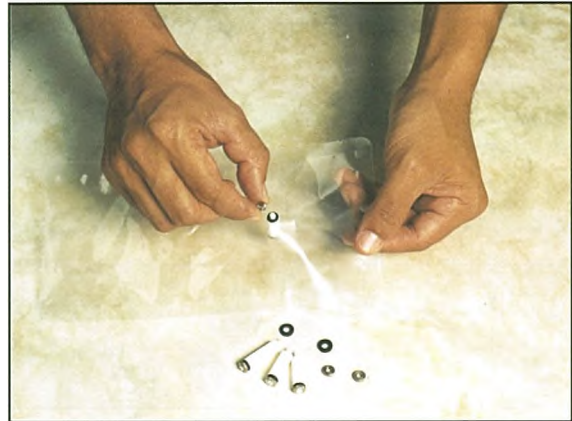
Fig.6 Insert and fix the packaging gland.
