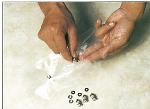
Fig.7 Insert and fix the probe holder
