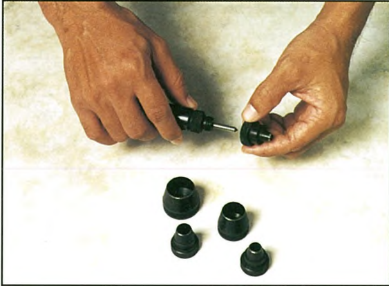
Fig 3 Select a suitable puncher head and fit into the puncher holder.
