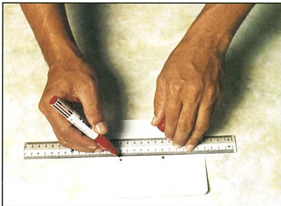
Fig.4 Mark 2 positions for punching.
