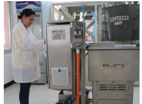
The dynamic settler used in microalgae production at AQD
