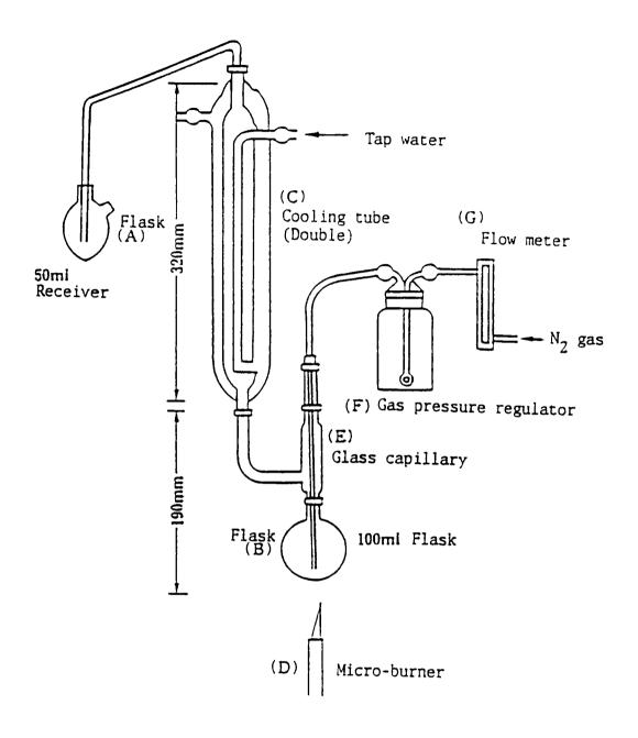
Fig. 1. APPARATUS FOR DISTILLATION (RANKINE METHOD)
