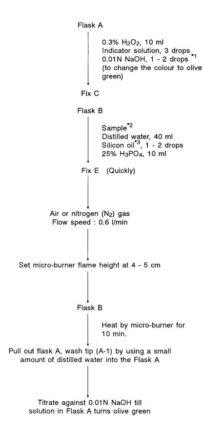
Fig. 2. Analytical procedure for the analysis of SO<sub>2</sub> by Rankine method.
