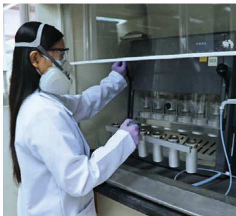
A chemist of AQD conducts a crude fat analysis that is part of the proximate analysis, one of the most requested analyses by academic institutions in Western Visayas, Philippines
