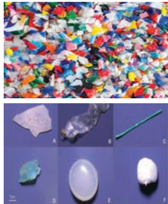
Figure 1. Microplastics (top) and their shapes (bottom): A - sheet; B - film; C - line/fiber; D - fragment; E - pellet/granule; and F - foam
