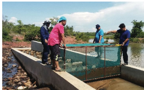
Fish passage construction at Hany Wang Chang Weir, Udon Thani Province, Thailand (left), and setting of fish trap at the exit pool of fish passage to observe its efficiency for fish migration (right)
