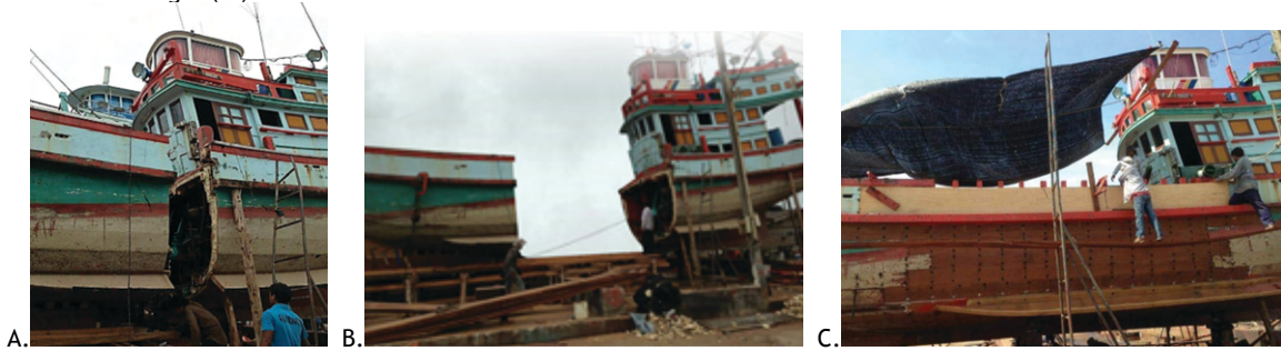
Box 11. Case study on improving the length of waterline of purse seiner in Thailand
