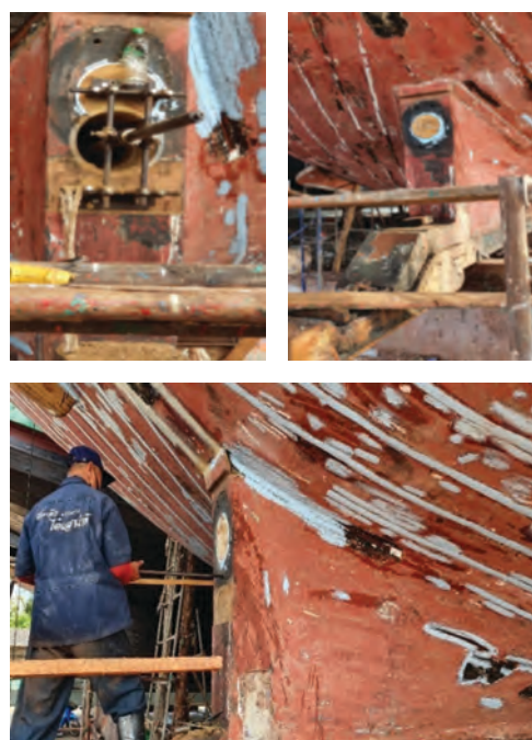
Figure 4. Refinement of the stern tube
