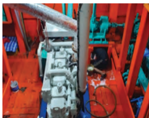
Figure 3. Installation of engine in the engine room
