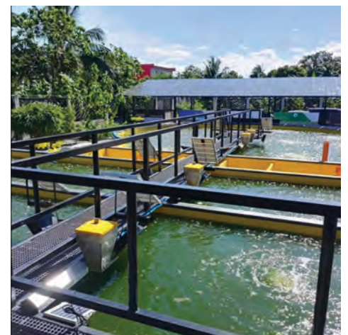
A modular aquaculture set-up with automated aeration, filtration, and nutrient system
