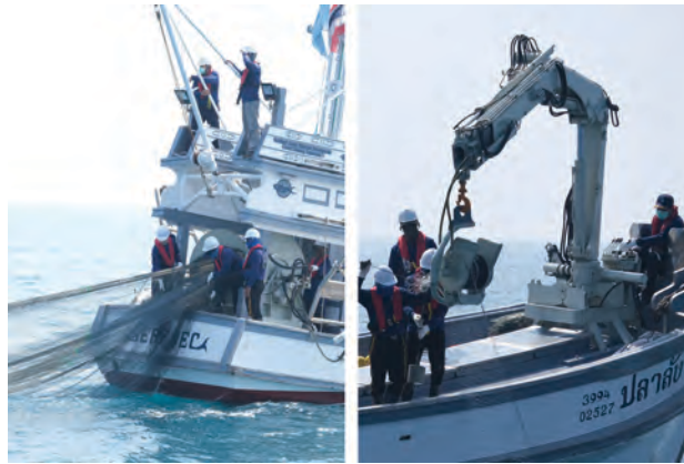
Equipment, i.e. net drum (left) and hydraulic crane (right), applied to reduce manpower onboard the fishing vessel
