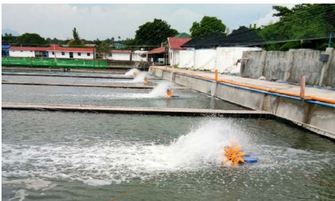
Use of paddle wheel aerators as a life support system for the shrimp in Taal, Batangas, Philippines
