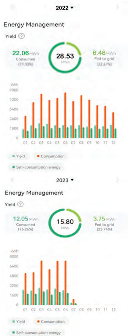
Figure 4. Power generation of the 20-kW hybrid solar energy system applied by SEAFDEC/TD in 2022-2023
