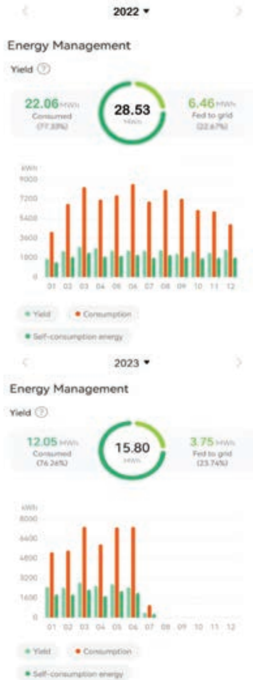
Figure 4. Power generation of the 20-kW hybrid solar energy system applied by SEAFDEC/TD in 2022-2023
