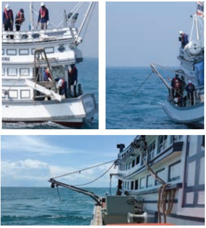
Figure 6. Adjustable U-shaped gallows of M.V. Plalung designed by SEAFDEC/TD
