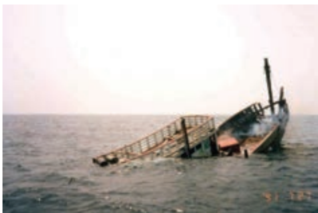
Figure 4. Derelict and confiscated wooden vessels were cleaned, punctured, and burned during the sinking process
