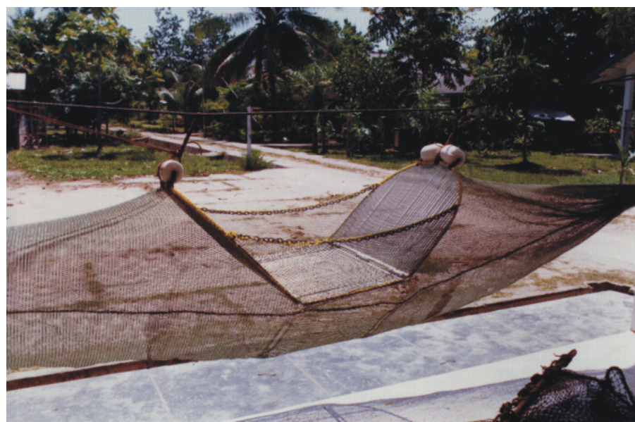
A new type of Juvenile and Trash Excluder Device, developed by SEAFDEC/Training Department
