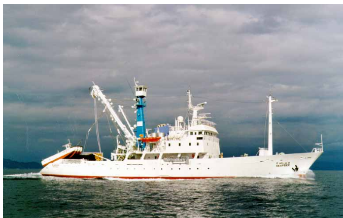
M.V. SEAFDEC, a 1178 GT purse seiner used for collaborative fishery resources assessment of the Southeast Asian waters as well as for regional shipboard training on fishing technology, marine engineering, navigation, and seamanship, and in the conduct of hydro-acoustic and fishery oceanographic surveys
