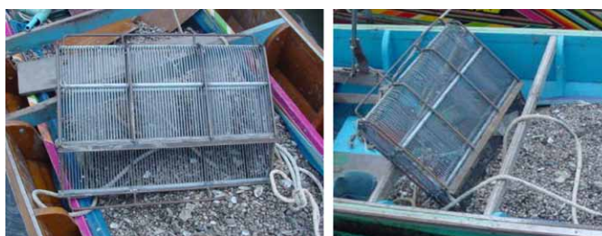
Fig. 9. Small size iron dredge in an outboard engine fishing boat
