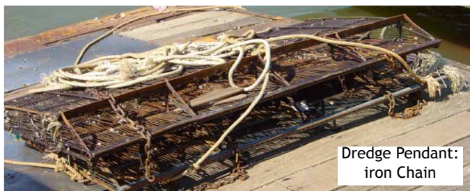
Fig. 8. Construction of iron dredge
