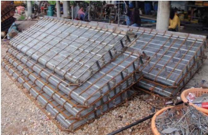
Fig. 11. Big-size iron dredge, entrance size 320 m Photo: Isara Chanrachkij
