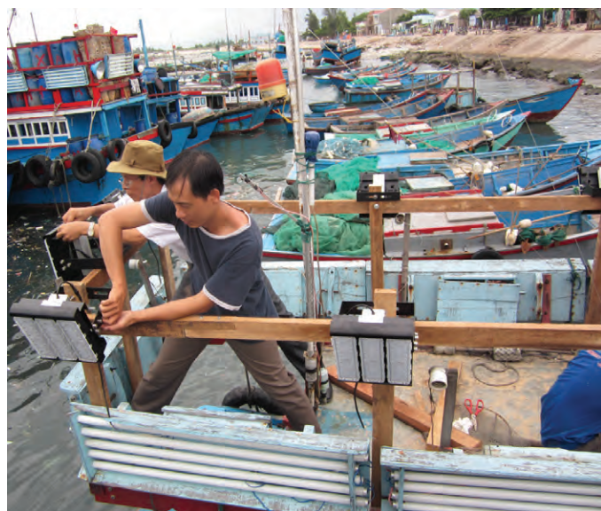
Installing LED light in purse seine vessels in Ninh Thuan, Viet Nam
