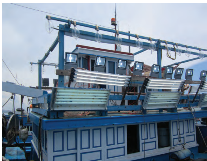
Purse seiners: (above) installed with common types of lamps (fluorescent bulbs and metal-halide lamps); and (right) installed with LED lights
