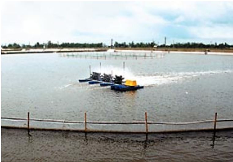
Fig. 6. The long-arm paddle wheel provides aeration and circulation
