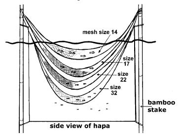
► The fingerlings that will be sorted are released on top of the sorter. This way, the fingerlings having a size smaller than the mesh size of the first sorting net will pass through to the next net in the series of sorters. The large size fingerlings will remain on the first sorter. Meanwhile, as the
