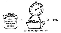
**Example:** A 5 x 10 m concrete tank holds 200 potential breeders that weigh 100 g each. The total fish biomass is computed as follows:
