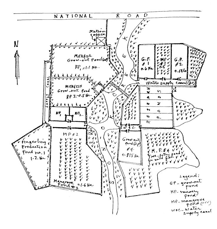
Fig. 2. Diagrammatic layout of Ubay Brackishwater Demonstration Farm, Son-oc, Poblacion, Ubay, Bohol, the Philippines
