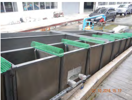
Fishway model (left) and preliminary experiments to monitor migration of indigenous fish species (right)
