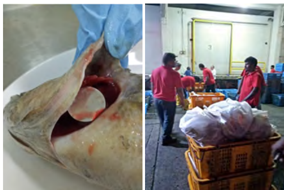
Button-type data loggers (left) for temperature monitoring in the cold chain pilot trials (right)
