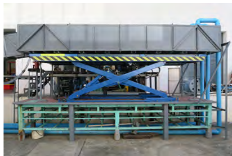
The slope of fishway model made adjustable from 5 degrees (left) to 11 degrees (right) using hydraulic equipment
