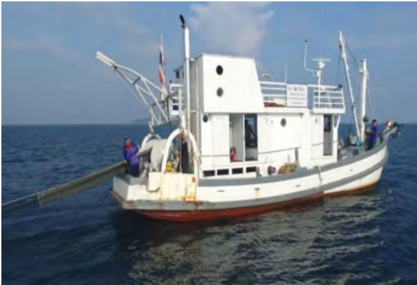
The M.V. PLALUNG equipped with facilities to improve crews' working condition, and net drum to minimize labor used in fishing operations
