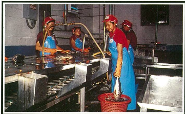
Segregation of rejected raw material
