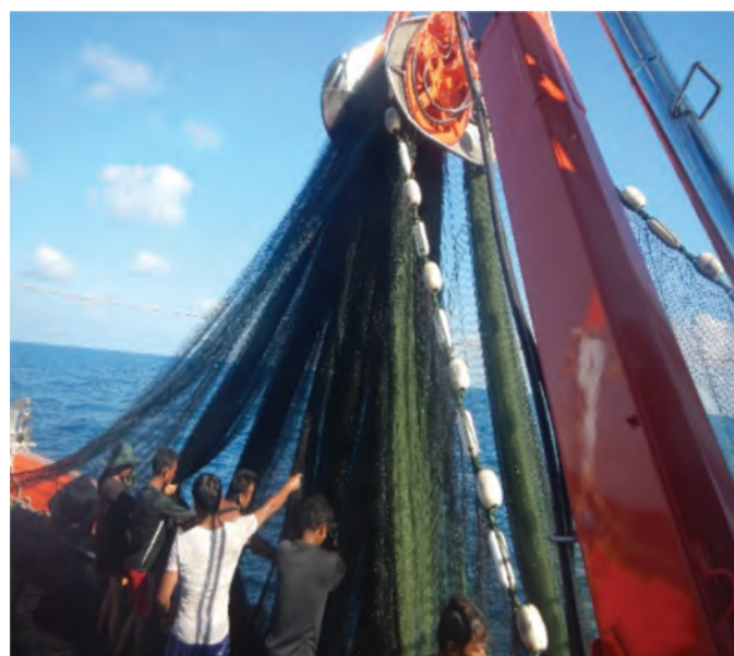
Figure 4. Hydraulic machinery (crane and power-block) to haul and stow nets reduces the number of manpower onboard fishing vessels
