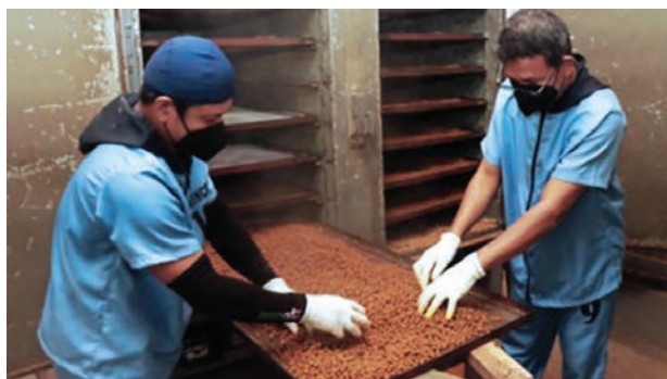
AQD feed mill workers spreading out the newly-formed wet pellets on a tray before placing them inside a dryer as part of the process to produce aquaculture feeds
