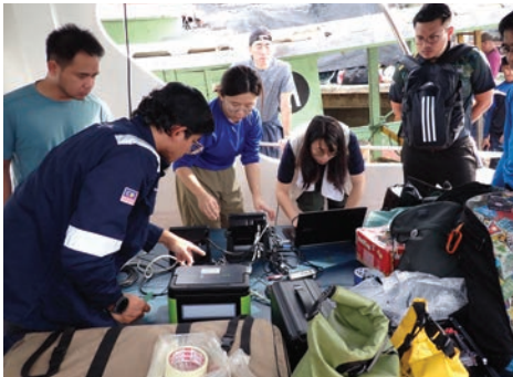
Testing the modified Furuno FCV-600 system portable echosounder for acoustic data collection in the waters around Pulau Kapas, Malaysia
